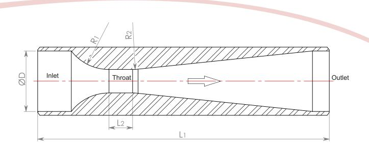
The Hydropneumatics critical flow venturi (CFV) is an excellent device for generating a known measured flow rate. The CFV exhibits a nominally linear relationship between inlet pressure and mass flowrate. A particular flowrate can be established by applying the proper value of inlet pressure. The range of available inlet pressure values will limit the range of flow rates that be generated.
