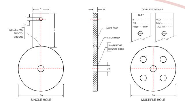
These Plates are similar to Square Edge Concentric Orifice Plates in construction, except, there is no bevel provided at the outlet face of the Plate. The Orifice Bore Diameter designed as per ISO 5167 / RW Miller.
